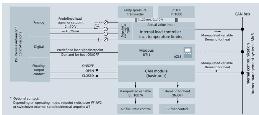
Output modulation and integration into LMV5 process automation
